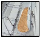
Large Roof Manhole has an "ob-round" shape and rotating latch for easy entry and exit.
